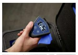
**PD-SGS** is a dual transducer PD detector for Switchgear. The instrument detects TEV signals generated by internal discharge as well as acoustic discharge generated by surface tracking or corona.
