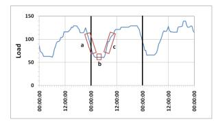
In some cases cable failures have occurred following load increases and in other cases following load a decrease. Determining a measure for the relationship between load and pd is another key factor to take account of in assessing circuit or switchgear criticality.
