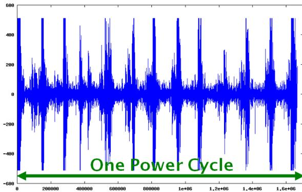
Figure 2: High noise levels detected by HFCT sensor (Vertical scale  $\pm 600\text{mV}$ )
