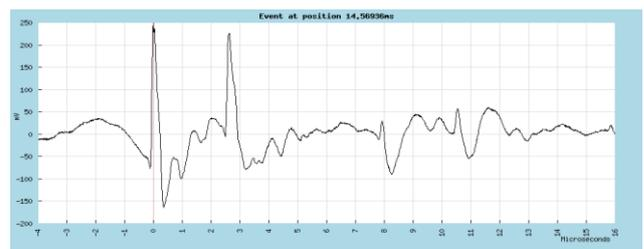
Figure 5: PD as displayed on web front end
